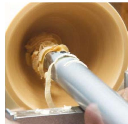
ABOVE: The size and the mass of the hollowing system makes deep hollowing a joy. Here, a shrouded cutter is being used
